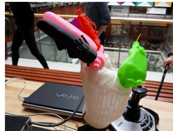
Figure 4: The 3D printed hand with customized movable fingers. Each finger was modified from a base model template by each participant team.
