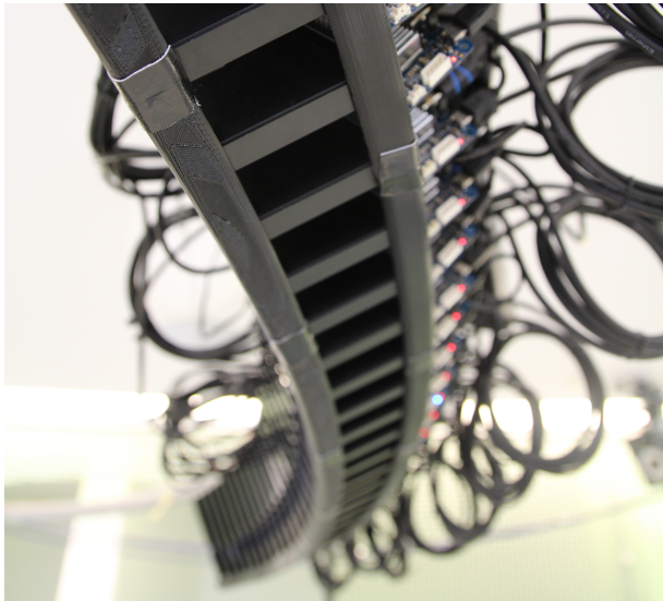
Figure 4. Projector rail with 45 projectors, each with an Odroid rendering board.
