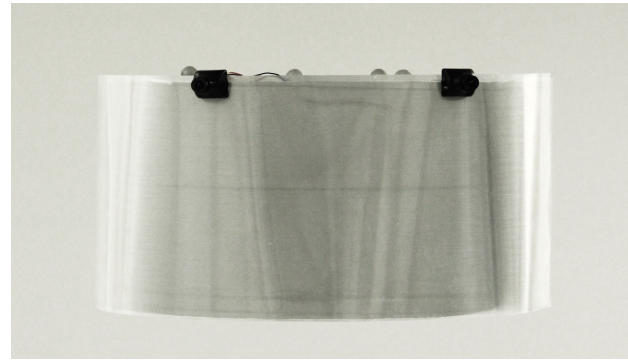
Figure 3. LightBee prototype with two cameras and retroreflective surface.
