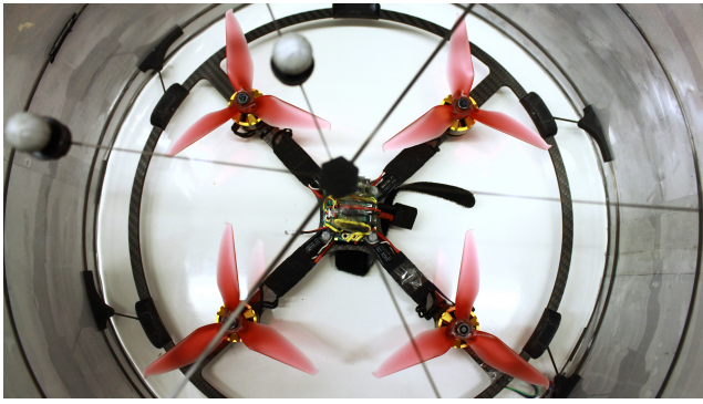
Figure 2. The LightBee prototype viewed from above. Special rotor blades direct airflow through the cylinder.
