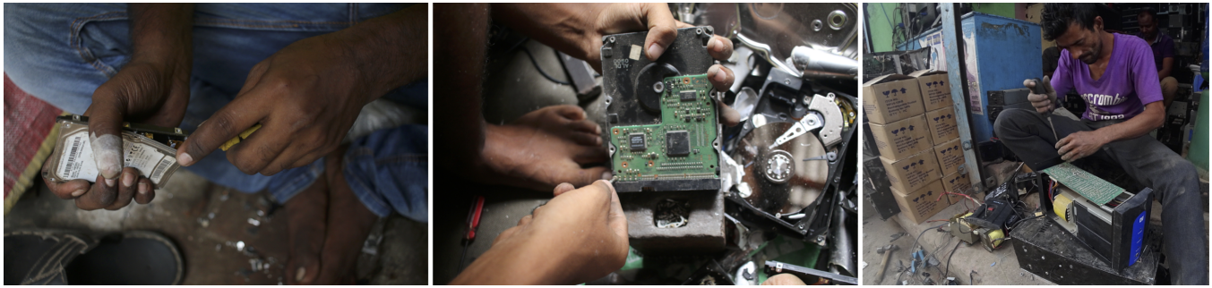
Figure 2: Handworks of bhangaris (from left to right): (i) a bhangari is opening a laptop hard disc with a knife; (ii) a bhangari is pulling out ICs from a mother board with a needle; (iii) a bhangari is breaking a computer motherboard.
