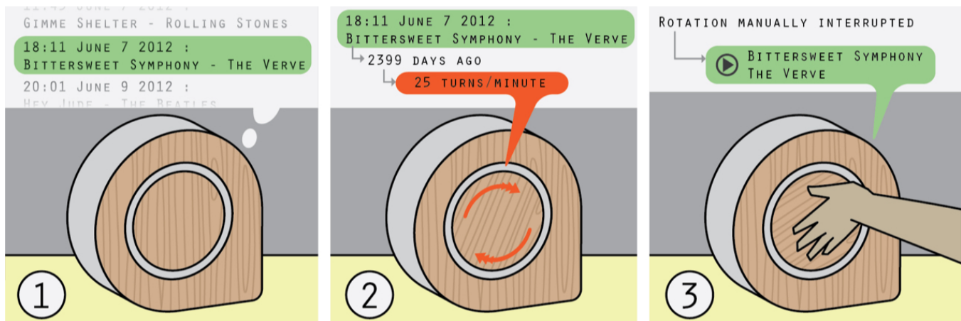
Figure 3: 1) Olly’s algorithm has a ‘success’ and it randomly selects a specific listening instance from its owner’s Last.FM library; in this case, the song Bittersweet Symphony that was listened to on 18:11 June 7 2012 is selected. 2) The internal disc begins to rotate indicating that a song is availability to be played; in this case, the listening instance is quite old which causing the disc’s rotational speed to be quite slow; 3) The user notices the rotation and manually spins the disc to trigger the song to play.
