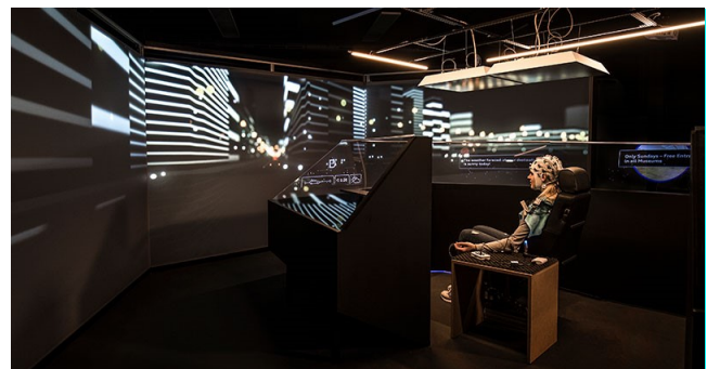
Figure 5: Experimental set-up: The participant is in the center of the prototypical car wearing the mobile EEG device and performing the visual concentration task (displayed on the front window screen) in the leisure-oriented condition (©Audi AG).
