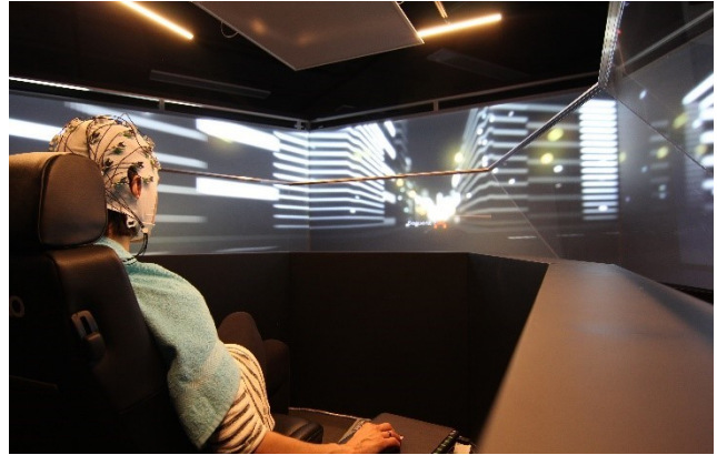
Figure 3: Lighting concept for the leisure-oriented configuration of the prototypical self-driving car: linear, darker light with very few blue components (©Audi AG).
