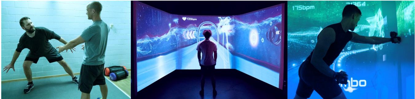
Figure 1: The ExerCube (middle, right) provides players with a playful full-body functional fitness experience that is on par with personal training sessions (left). The player is surrounded by three walls, which serve as projection screens and a haptic interface for energetic bodily interactions. Movements are tracked with two HTC Vive trackers attached to players' wrists.
