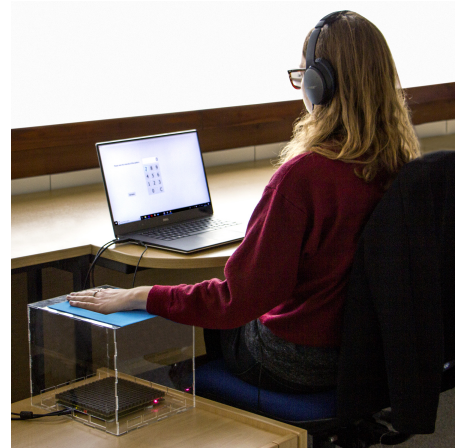
Figure 3: The set-up for the user studies. Participants were perceiving the mid-air tactile pattern on their left palm while rating each pattern on a designated laptop.
