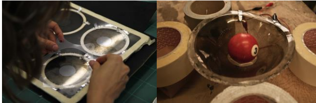
Figure 8. Placing acrylic frames and testing weight-based stretch.
