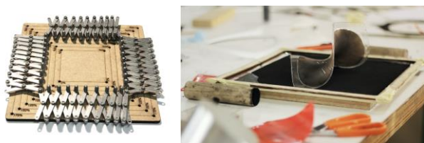
Figure 4. Stretch mechanism with scale guide, foam applicator with DEMES EAP
