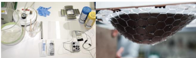
Figure 5. Materials and tools for silicone EAP fabrication and a silicone HAP actuator with a supporting structure molded into the membrane.
