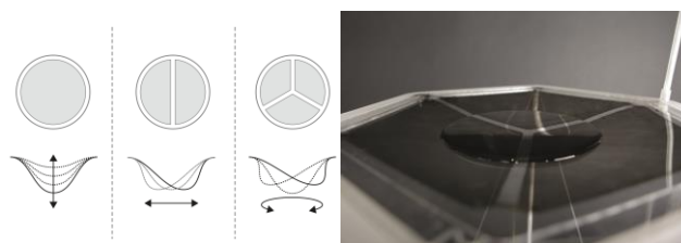
Figure 3. A HAP actuator with additional movement axis, demonstrated in Fluid Morphologies [9]. Seen in motion in https://vimeo.com/163376887
