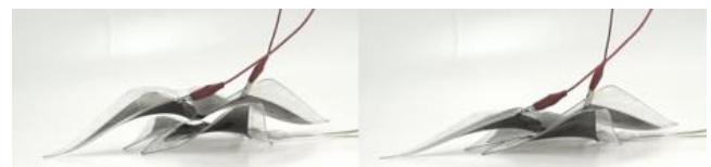
Figure 11. Two connected “dancing” EAPs. See motion at vimeo.com/106512539
