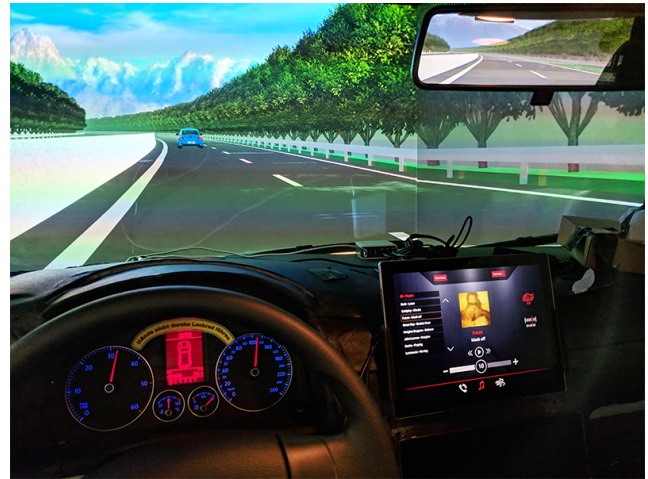
Figure 1: Study setup showing the driving scenario and an example of the IVIS used to investigate the interaction between UX and trust.
