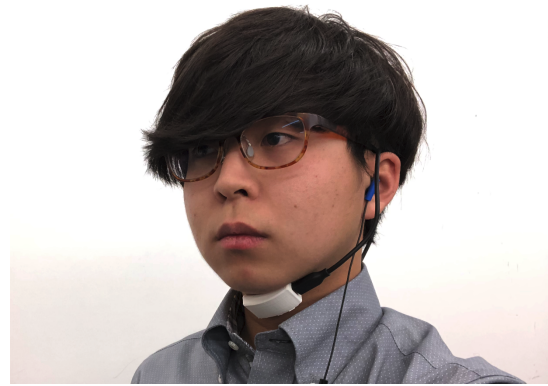
Figure 11: Future Image: possible configuration of an ultrasonic probe and an open earphone
