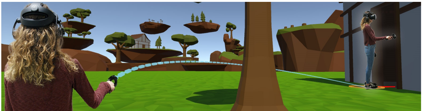
Figure 1: A user is teleporting herself in a Virtual Environment using the Curved Teleport . It allows her to teleport around an obstacle and graphically choose the orientation, which she wants to face after teleportation only by using the curved trajectory visualization with orientation indication, and without having to turn her body in the physical world.
