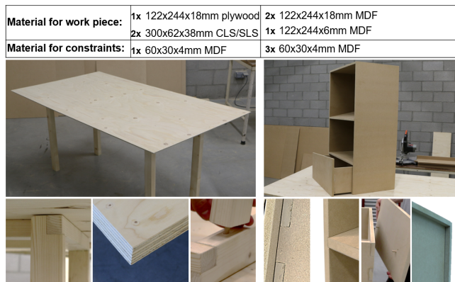
Figure 16: Several constructions fabricated with JigFab, including a table and a display cabinet with drawer.
