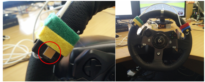
Figure 1: Thermally-enhanced steering wheel with small Peltier elements.
