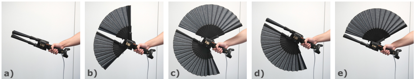
Figure 1: The five states of our shape-changing haptic VR controller Drag:on investigated in our user study. a) shows the device state S_{closed} with minimal surface area. When increasing its surface area symmetrically as shown in b) ( S_{half} ) and c) ( S_{full} ), the controller adapts its drag and mass distribution to provide different haptic sensations during VR interaction. If opened asymmetrically on the d) left ( S_{left} ) or e) right ( S_{right} ) side, torque is induced when moving the controller.
