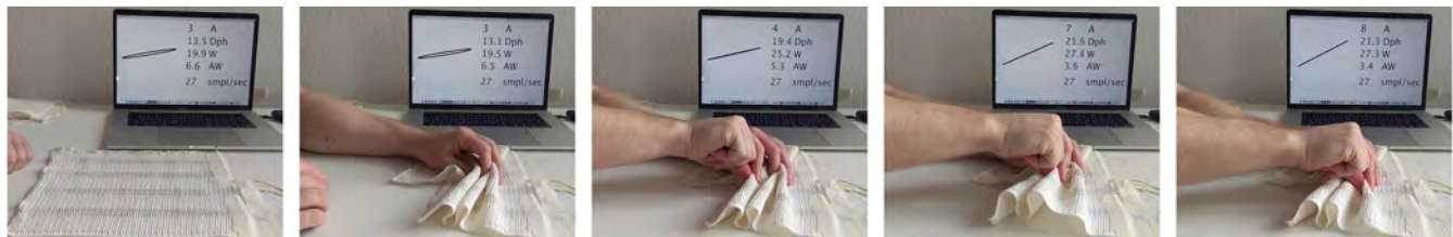
Figure 1: Using Teksig to reliably identify pinching on a wrinkled textile.
