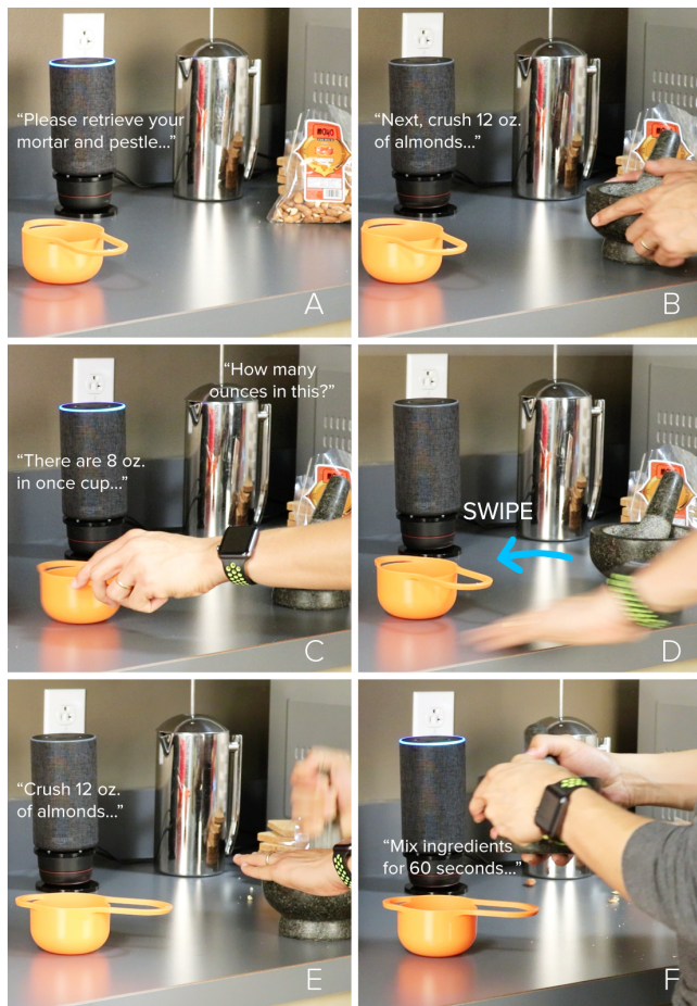
Figure 9. Recipe helper demo application. When a recipe is loaded, the system asks the user to retrieve necessary items (A), moving to the next step automatically upon detection (B). Contextual questions such as “how many ounces are in this” after putting down a measuring cup are possible (C). Swipe gestures move between recipe steps (D & E). When a user is finished with a step (e.g., mortar and pestle lifted from surface), the recipe can automatically advance (F).
