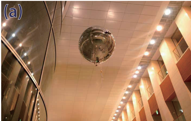
Figure 1: Our prototype: (a) ZeRONE is flying indoors. (b) The user can touch our blade-less drone without fear or injury.
