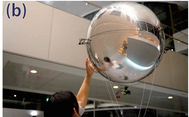
Figure 1: Our prototype: (a) ZeRONE is flying indoors. (b) The user can touch our blade-less drone without fear or injury.
