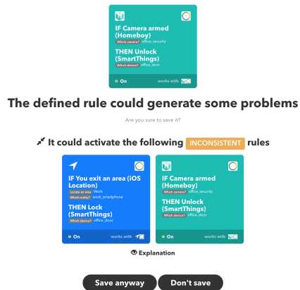
Figure 4: The Problem Checking interface showing an inconsistency between an already existent rule and the defined one.
