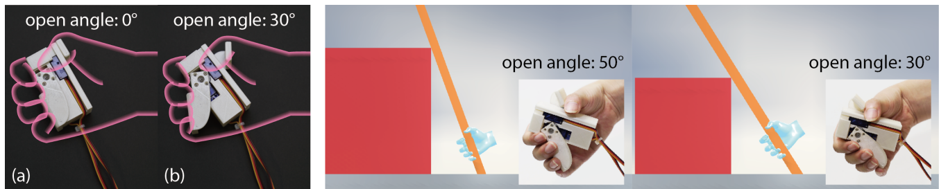
Figure 1: (left) PaCaPa is a handheld device with two wings that open (a) and close (b) to render a sense of pressure on the palm and fingers when the virtual tool in a user's hand makes contact with virtual objects. (right) Our device can render a target object's size with different open angles when the hand is wielded in the same way.
