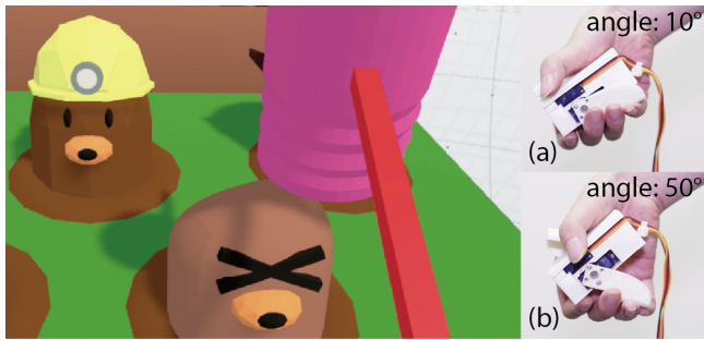
Figure 12: (left) Whack-A-Mole application that highlights stiffness and shape. (right) When a user wields the stick in the same direction, the specific angle is presented when (a) soft / (b) hard mole is hit.
