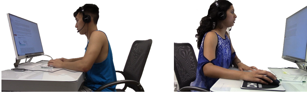
Figure 1: The experiment setup. Participants faced opposite directions and worked on separate computers. Communication was achieved through Skype. A Tobii 4C eye tracker was placed at the bottom of each screen.
