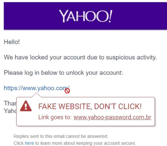
Figure 1: Our link-focused phishing warning with forced attention. The warnings appears when a user hovers over a phishing link. The warning uses sparse text and draws attention to the link’s actual URL in order to facilitate its inspection. We further force a user’s attention to the warning content by deactivating the link in the email when the warning appears (and mouse cursor turns into a “no” symbol), forcing the user to click the URL displayed in the warning if they choose to proceed.
