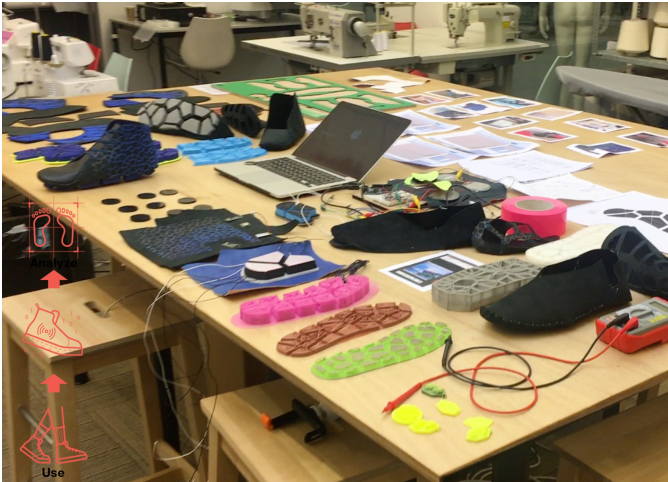
Figure 7: A selection of the several samples developed to create electronic and mechanical sensing inside the structure of the shoe soles.
