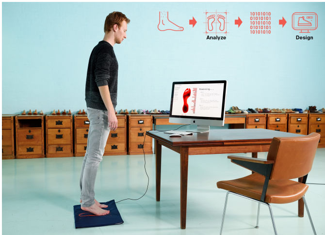
Figure 4: The SoleScan pressure pad and software recorded footstep size and pressure. Photo by Bart van Overbeeke
