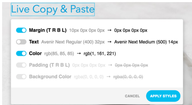
Figure 2: Poirot allows copying styles from one element and pasting the styles to another element. The resulting window lets designers toggle on and off properties to see a live preview of what styles are being transferred.
