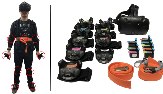
Figure 1: Left: Participant wearing all nine HTC Vive trackers and headset (highlighted by red circles). Right: HTC Vive trackers, headset, and accompanying devices.
