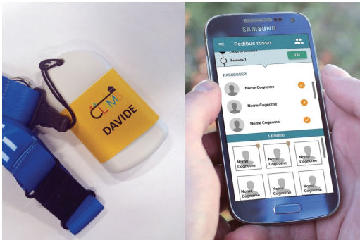
Figure 2: The proximity detection BLE device given to children (left), which connects to the mobile application installed on the volunteer's smartphone (right).
