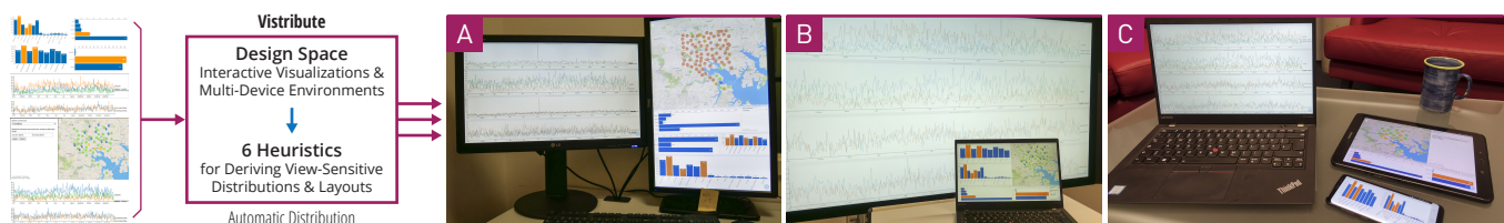
Figure 1: The Vistribute system: Based on a design space we derived six heuristics that can guide an automatic distribution of visualizations in changing device setups, e.g., (a) dual desktop, (b) laptop and large display, or (c) mobile device ensemble.
