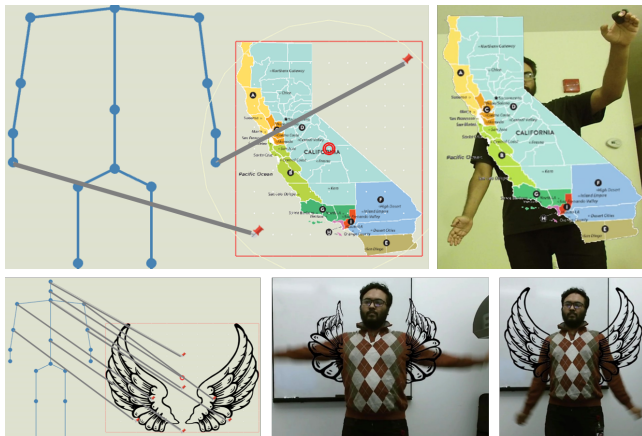
Figure 10: Deformation examples. Top: manipulating a map by two hands. Bottom: flapping wings via arm motions.
