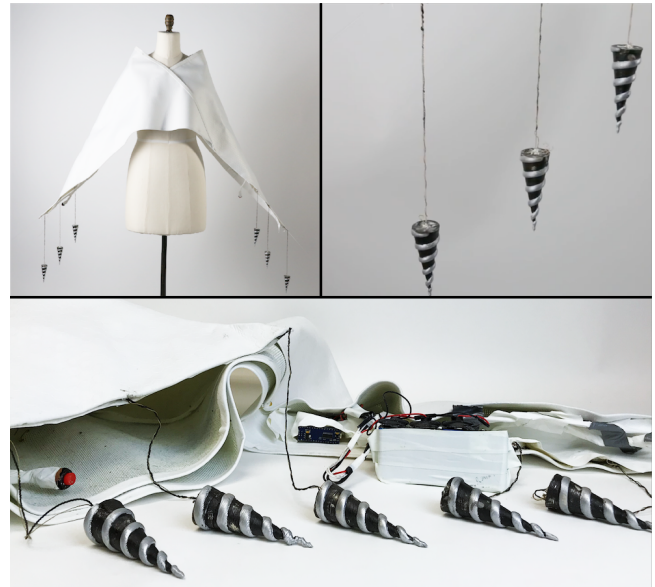
Figure 13: Active garments triggered by 2-ply shrinking thread actuators.
