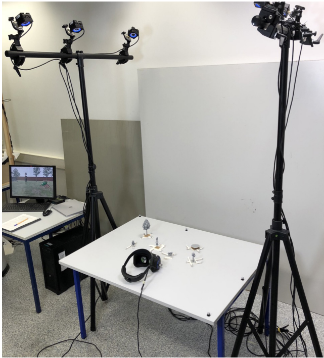
Figure 2: System setup with three Optitrack cameras on each side of the table and HMD and tangibles on the table.
