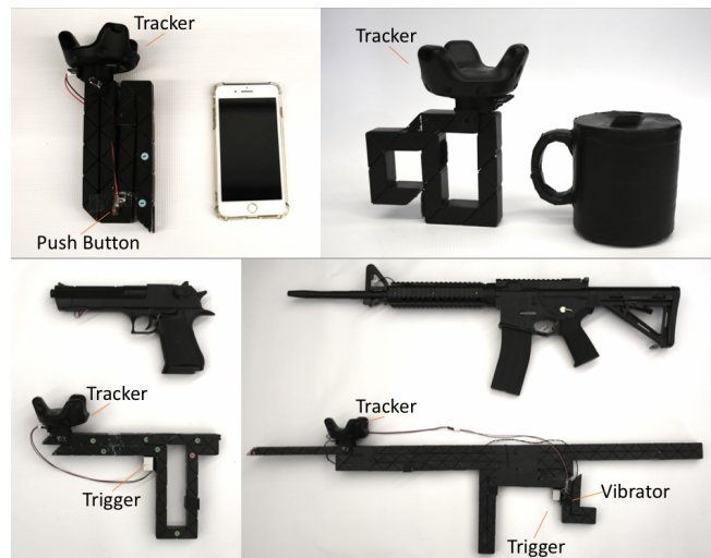
Figure 15: HapTwist-generated Proxies and their real-object counter parts.
