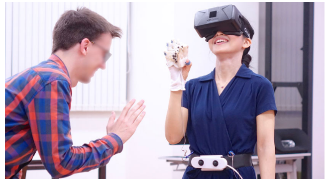
Figure 1: We explore a wearable visual device that allows a user to change their body representation, in realtime, to that of a small-person
