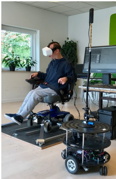
Figure 11: Controlling a telerobot with the wheelchair. The camera on top of the robot transmits a full, immersive, 360- degree view to the operator who drives it with the wheelchair joystick.
