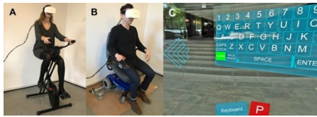
Figure 7: (A) Participant on bicycle locomotion device with VR headset; (B) Participant on wheelchair locomotion device with VR headset; (C) Parking-mode, showing the panning view of the real scene with keyboard tool activated; keyboard- and driving-mode buttons are located in the lower part of the field of view. All buttons can be activated with gaze and head input.
