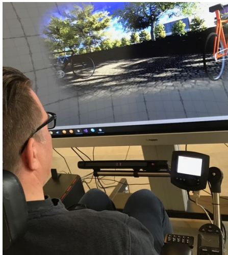
Figure 8: Gaze-driving a wheelchair while looking at a large monitor. A remote gaze-tracker is mounted on the wheelchair in front of the user.
