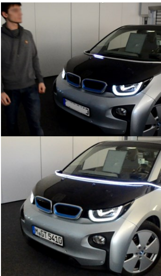
Figure 5: “Light-belt”: an intent-based 360° communication (top: reflecting detection of a pedestrian via a moving light segment in the “light-belt”, bottom: fully pulsing “light-belt” without reflecting detection).
