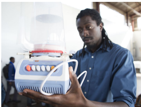
Figure 8: The team that won the prize for most frugal design built a centrifuge from a food mixer. Photo credit to Jeffrey Barbee/Alliance Earth
