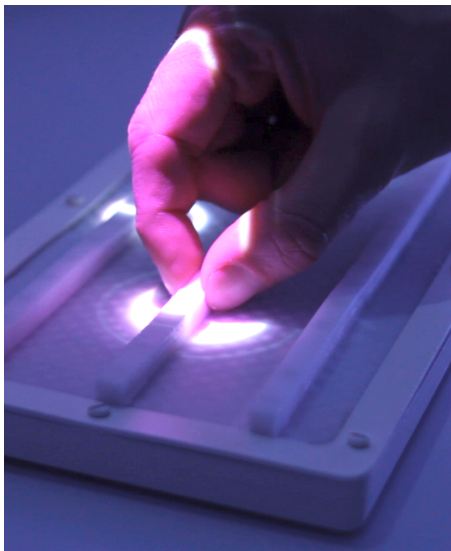
Figure 1: StringTouch combines features of touch screens with haptic elements. Along three silicone ridges the user can perform gestures and deform the material in inwards and outwards direction.
