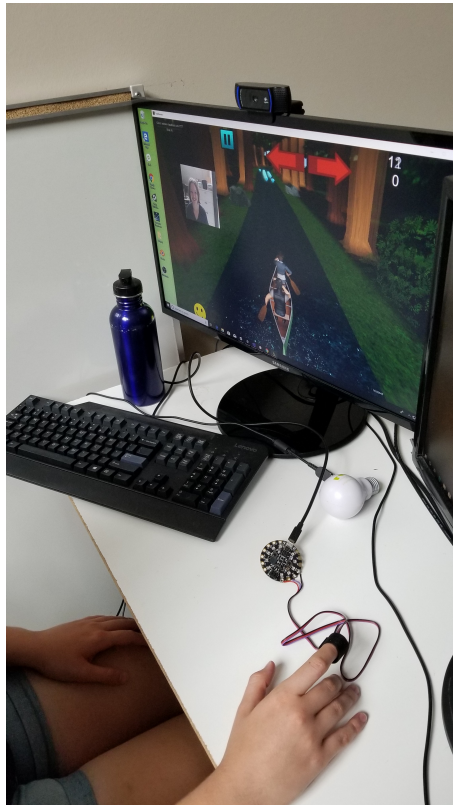
Figure 3: Game setup: Webcam, circuit playground attached to finger, and game on screen.
