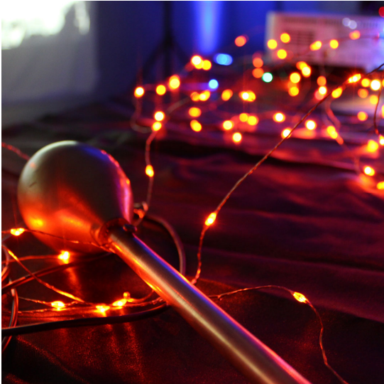
Figure 4: A Close up of one of the maraca controllers that ensures players hold hands throughout play. If contact is broken, the wave of life disappears from the screen and play cannot resume until the players reconnect their hands.
