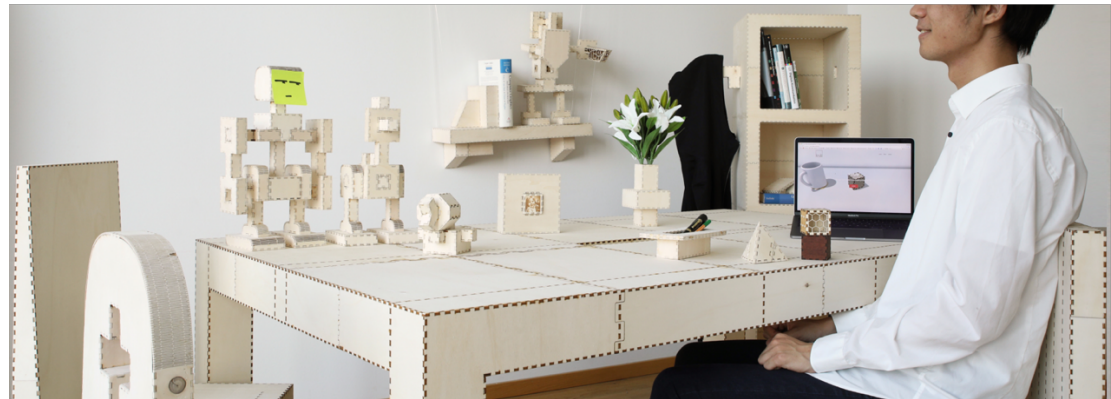
Figure 1: A selection of objects created using kyub , a software system that allows users to design 3D objects for laser cutting. By affording closed box structures, objects made using kyub are very strong. This allows users to make tables, shelves, and chairs that can hold a person. (All shown objects are assembled from 4mm plywood sheets—pressure fit, not glued).
