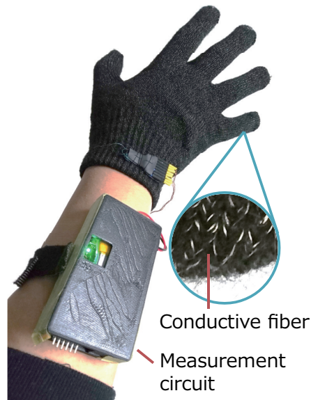
Figure 1: Grov prototype. The white strings are conductive fiber. The weight of the device is 70 g including the circuit and battery; the glove part weights 17 g.
