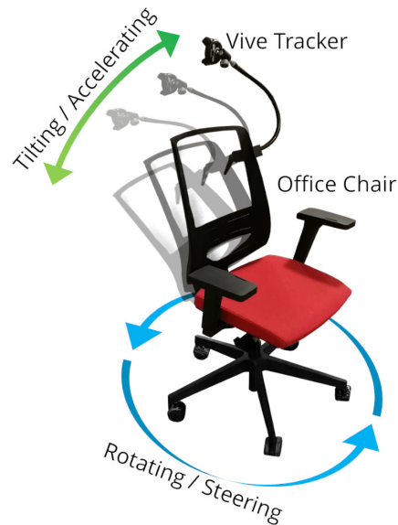
Figure 2: The mapping of a regular office chairs' movement onto our VRChairRacer racing cart. An HTC Vive Tracker is used to recognize the chair's position and for accelerating through tilting the back. Rotating the chair is used for steering.
