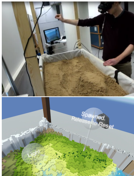
Figure 2: External view on a user interacting with VRBox (top) and his view in the tabletop perspective mode. The user is performing a pouring gesture to place virtual objects in the environment.
