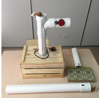
Figure 2: Pusing Tiang can be disassembled into three parts for easy transportation.
