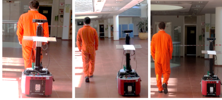
Figure 1: The robot's following angles: 0° (left), 60° (center), 90° (right)
