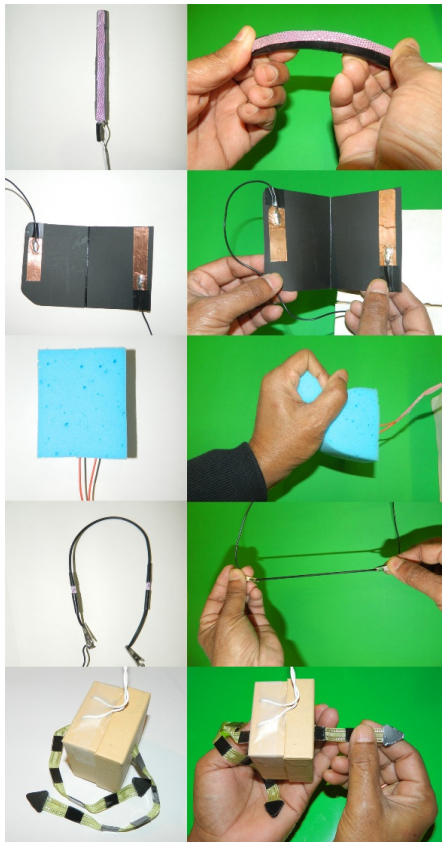
Figure 2: Sensor-enabled set of artifacts (left) and the associated tangible manipulations (right) viz. bend, fold, squeeze, stretch and pull (top to bottom).
