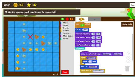
Figure 3: A Pirate Plunder level that requires a custom block with two inputs (parameters) and cannonball sprite cloning.
