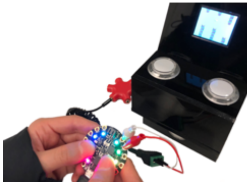
Figure 5. Buttons from an Adafruit Circuit Playground Express (CPX) used as a controller for the Flappy-bird game. The CPX is coded using blocks (and a custom plug-and-play headphone-jack bus protocol) within MakeCode Maker. On MakeCode Arcade, a user simply programs additional buttons using our packages, which are auto-detected when plugged into the headphone jack hub.
