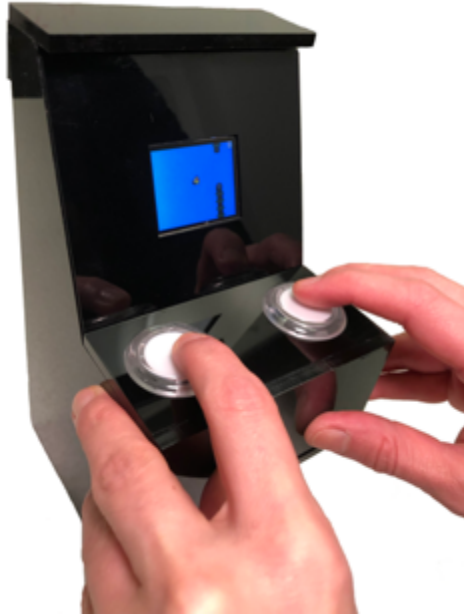
Figure 1. An example of a completed MakerArcade system in the form of a miniature Arcade Cabinet running a user-created Flappy-bird like game with a default set of buttons mapped. This game (and others) can be mapped to different sensors (like an accelerometer) that a user can program and map as an alternative controller that is plugged into the cabinet which contains a headphone jack and uses our custom headphone jack-based hardware protocol.
