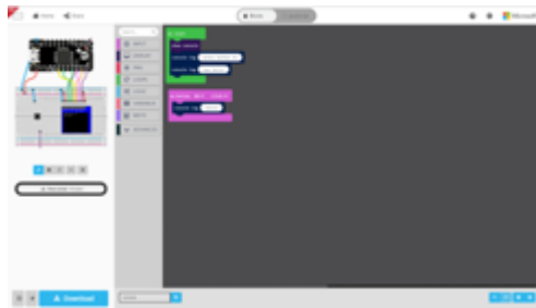
Figure 3. Microsoft MakeCode Maker (beta) that allows a user to program and prototype electronics. We provide packages which show a user how to physically create an arcade (with a screen) and buttons mapped to a microcontroller. We also provide mappings on how to create additional plug and play components (for custom controllers, sensors or modules), that use a custom headphone jack-based hardware bus protocol. These mappings when programmed by a user, are auto-detected when plugged into our MakerArcade system.
