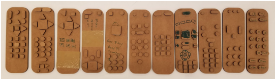
Figure 5. Eleven remote-control prototypes created by P10-P20 using the cardboard toolkit. While many contain similar layouts as standard remotes, there are significant differences in button placements across participants.
