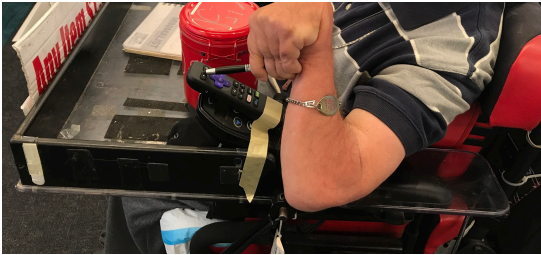
Figure 2. Picture of wheelchair user's technique to improve accessibility of commercial remote-controls (taping a television remote next to their joystick).
