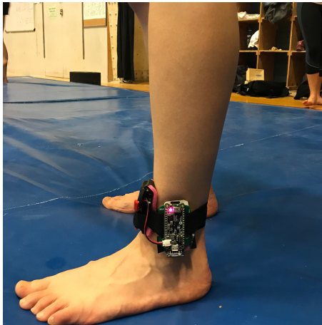
Figure 2: The AUFLIP sensor is worn on the ankle, purposefully offset from the center of mass; flips that are not ballistic often are the result of a non-stiff body.
