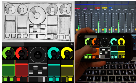
Figure 4: User-defined 2D interface created with TouchOSC based on a drawn sketch.
