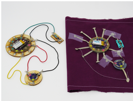
Figure 1: Craftec Version 1: Hard (left) and Soft toolkits (right).
